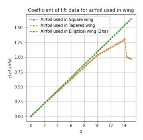
The above charts are just used for testing. You can see the square UAV wing that is used in the UAV, plus of the coefficient of lift, comparing  $2\pi\alpha$  to the coefficient of lift data given in the assignment for NACA0012 as a sanity check.
