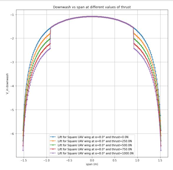
Given that the downwash directly impacts the effective angle of attack, and hence coefficient of lift, the downwash distribution across the span of the wing has the same shape as the local coefficient of lift curve.
