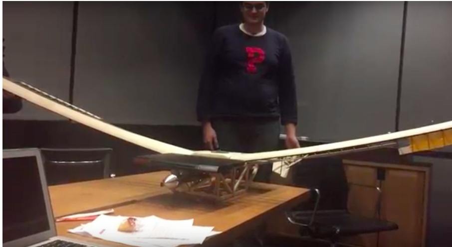
Figure 8.1.2.1: Two team members lifting up the aircraft for the wingtip test while using laptops to simulate the expected weight
